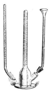
"The general form" of Dr. Doremus' apparatus is not new; it is a Cooper's mercurial receiver, known since 1825, with a bulb blown near the mouth. Neither is the graduation of the tube for the direct reading of the proportion of urea new. This graduation, to which I will revert, was first suggested by Russell and West (Journal of the Chemical Society, XXVII, page 749), and more recently by A. W. Gerrard in the Pharmaccutical Journal (III, 464).
